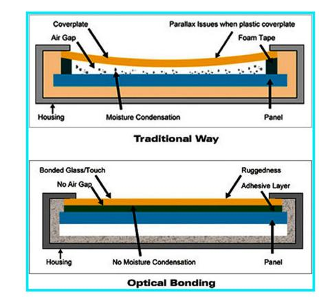
In a very simple display there are often three or four layers of glass and plastics, and a more complex display may have seven or eight layers. As light passes through each layer, there will be changes in the refractive index, resulting in some form of reflection.
